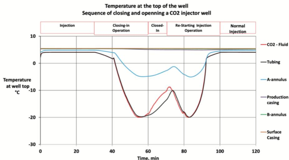
Figure 4. Temperature at different well elements in the top of the well for the sequence of closing-in a well after a long term injection period, well closed-in for a short period of time and re-starting injecting for a low reservoir pressure case (2750psi - ~ 190bar). CO<sub>2</sub> injection rates during the closing-in and the re-starting operations are proportional with time.
